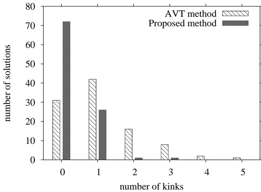
Fig. 2. Number of kinks in each solution for instance bier127.
